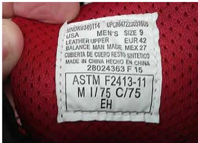
Look for this tag in the shoe. Notice the “ASTM F2413” and “I/75 C/75” ratings. These signify that the shoe is rated for impact and compression under the ASTM standard.
